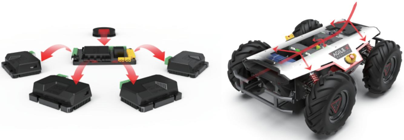
A bus interface is reserved around the body, and the top design with standard aluminum profiles is convenient for customers to match and access a series of external equipment such as differential GPS, binocular camera, laser radar, infrared/ultrasonic obstacle avoidance sensor, etc., allowing customers to complete customized in-depth secondary development.
