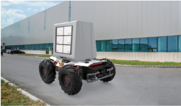
Based on SCOUT chassis and self-driving technology, with laser scanner, binocular camera and ultrasonic sensor to construct multi-sensor fusion navigation system, it can complete timely and accurate logistics delivery task in semi-closed environment such as park, factory area, etc., realize unmanned operations, reduce manpower input and improve logistics efficiency.
